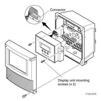
Figure 10.1.2 Display Unit Assembly
